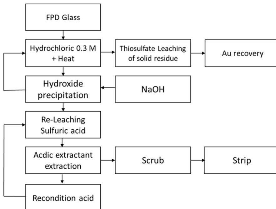
Figure 2. Treatment process flow-sheet for FPD crushed glass (CG). This recovers gold and indium.
