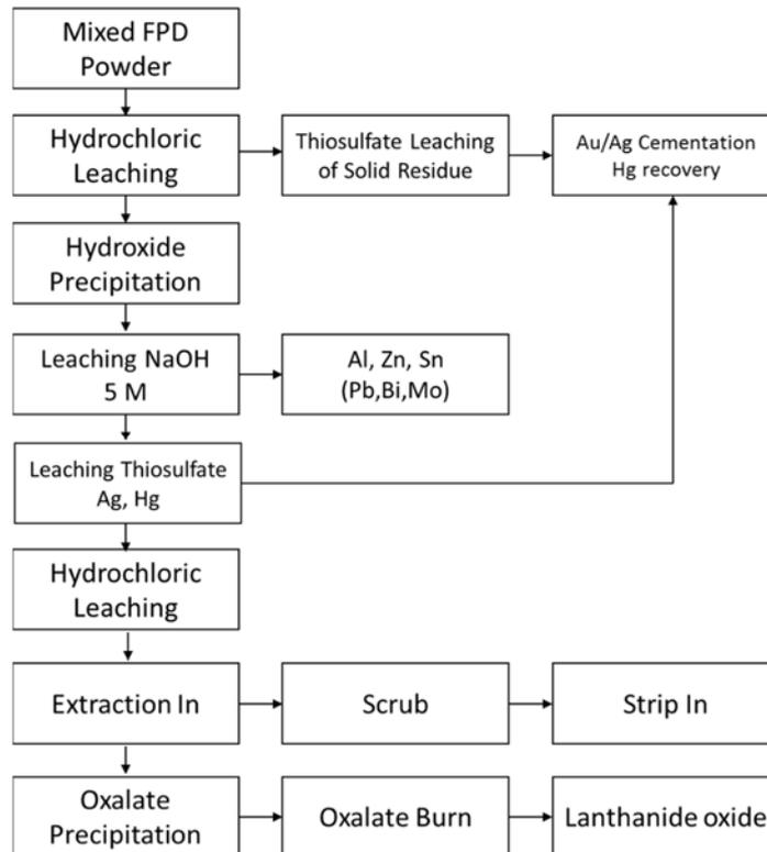
Figure 1. Treatment process flow-sheet for a fine fraction of mixed FPD powder (MP). This recovers gold, silver, rare earths and indium (simplified, there can be some purification steps excluded).
